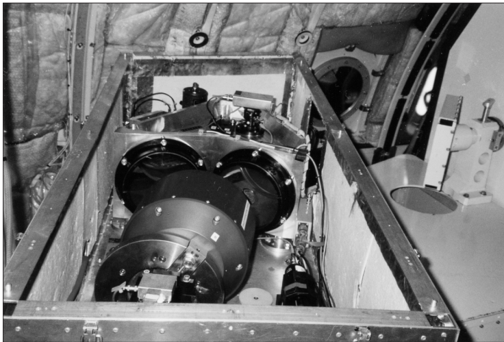
Fig. 2. Optical set-up of the MIROR spectrometer installed in one of DLR's research aircrafts.
