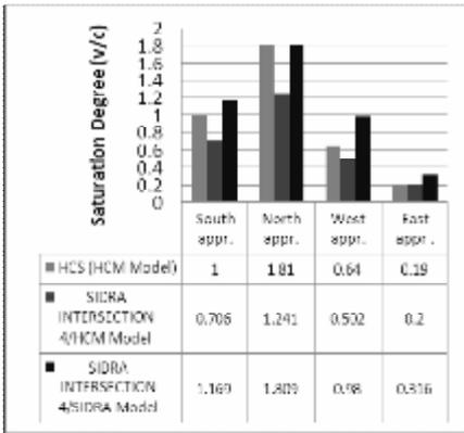
Figure (13) Saturation Degree (v/c) per Approach\Palestine Street Intersection 2 (at off Peak Hour)
