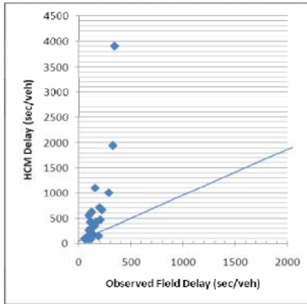
**Figure (20) Observed field delay versus. Theoretical delay (SIDRA INTERSECTION 4/SIDRA Model)**
