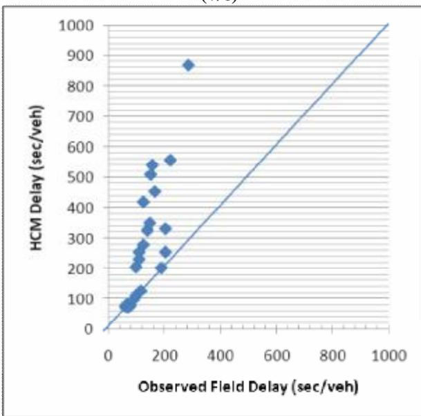
Figure (18) Observed field delay versus Theoretical delay (HCM Model)
