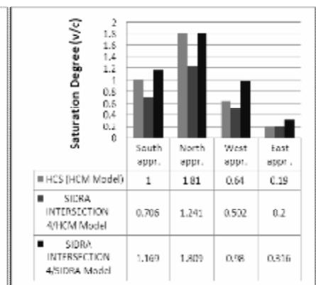
Figure (12) Saturation Degree (v/c) per Approach\Palestine Street Intersection 2 (at Peak Hour)
