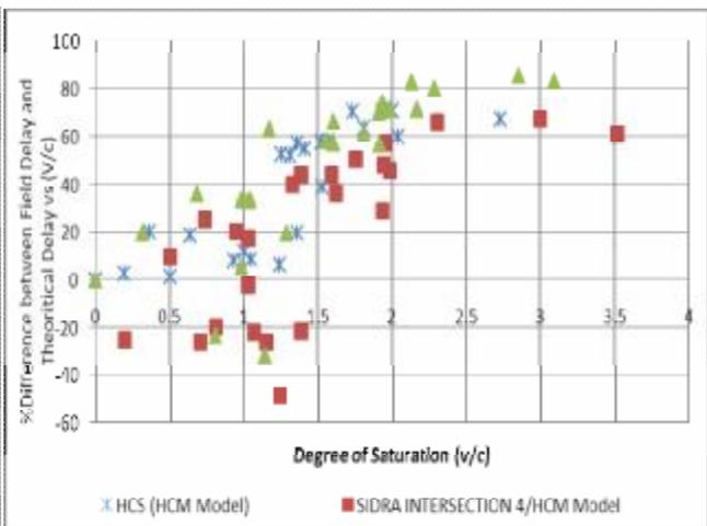
Figure (17) The differences between field delay and theoretical delay computed by the three models according to degree of saturation (v/c)
