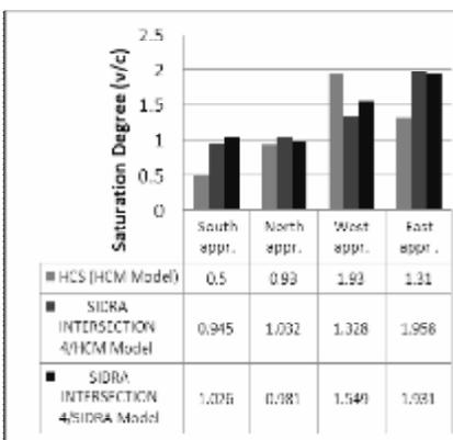
Figure (10) Saturation Degree (v/c) per Approach\Palestine Street Intersection 1 (at Peak Hour)
