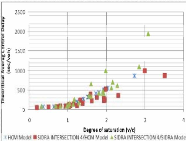
Figure (16) Theoretical delay calculated by the three models according to degree of saturation (v/c)
