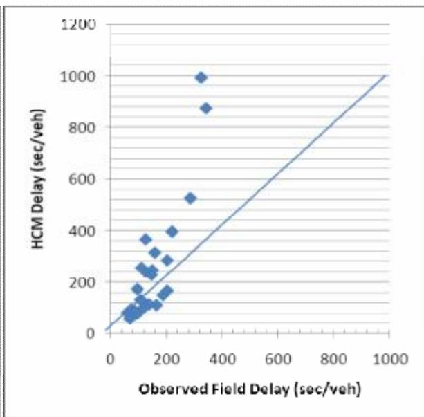
Figure (19) Observed field delay versus Theoretical delay (SIDRA INTERSECTION 4/HCS Model)
