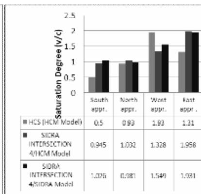
Figure (11) Saturation Degree (v/c) per Approach\Palestine Street Intersection 1 (at off Peak Hour)
