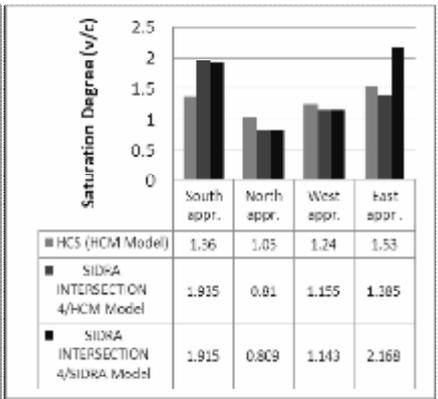
Figure (15) Saturation Degree (v/c) per Approach\Art College Intersection (at off Peak Hour)
