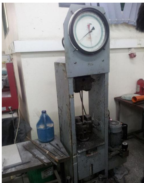
Fig. 2 Tensile test of steel bars
