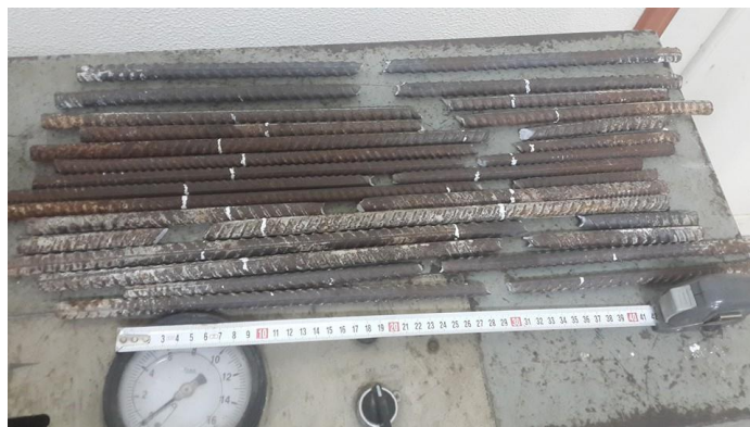
Fig. 4 Samples after tensile test
