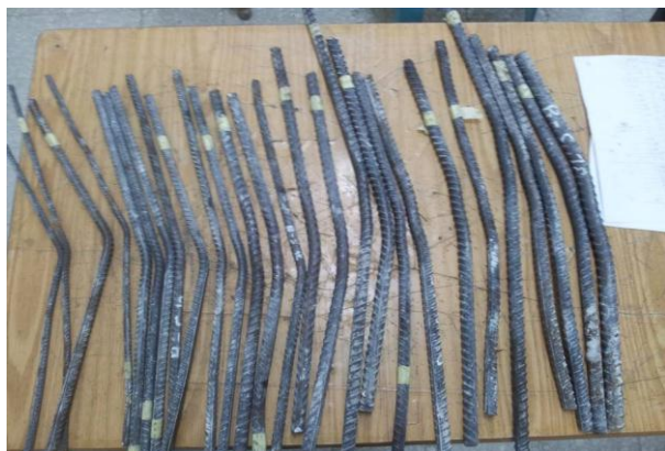
Fig. 5 Samples after bend & re-bend test
