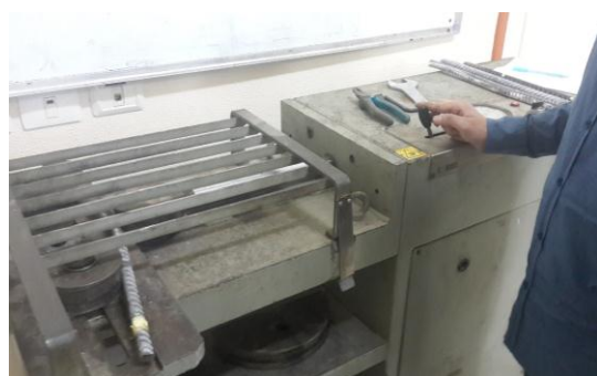
Fig. 3 Bend and re-bend test
