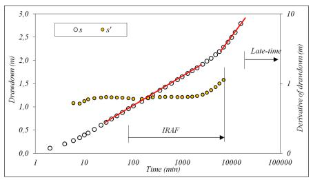
**Figure 1.** Graph showing drawdown (s) on primary vertical axis against time on a semi-log axis and derivative of drawdown (s') on secondary axis against time on a log-log axis
