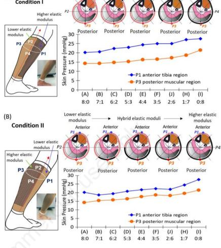
Figure 1. Skin pressure exerted by HCSs with nine types of hybrid elastic moduli. A) Condition I: segments with higher elastic moduli (shorter stretch) at anterior side, and segments with lower elastic moduli (longer stretch) at posterior region; B) Condition II: segments with lower elastic moduli (longer stretch) at anterior side, and segments with higher elastic moduli (short-stretch) at posterior calf.
