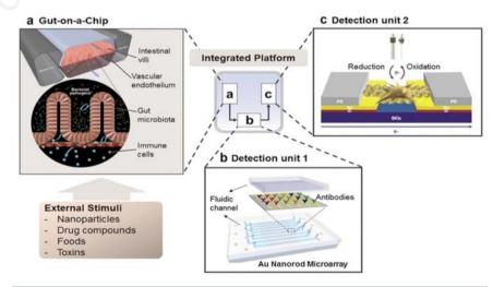
Figure 7. Concept of all human organ-on-a-chip. Advances in biomimetic micro engineering enable different organs features could be replicated on CHIP and to be integrated into a single micro device. Each further connected with each other via microfluidic circulatory system mimicking physiologically relevant functions as an *in vitro* model with complex, dynamic process into human body. Reproduced from ref.<sup>131</sup> with free use Creative Commons Attribution 4.0 International License.
