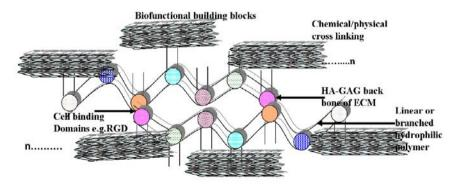
Figure 4. Schematic plan showing hyaluronan-GAG-core protein cross-linking strategy to design hydrogel based artificial skin-ECM analogue. Fundamental design includes HA-GAGs backbone that supports nanoscale protein-carbohydrate monomer buildings blocks pegged meticulously to mimic biostructure (n: repeating units; authors personal communication).
