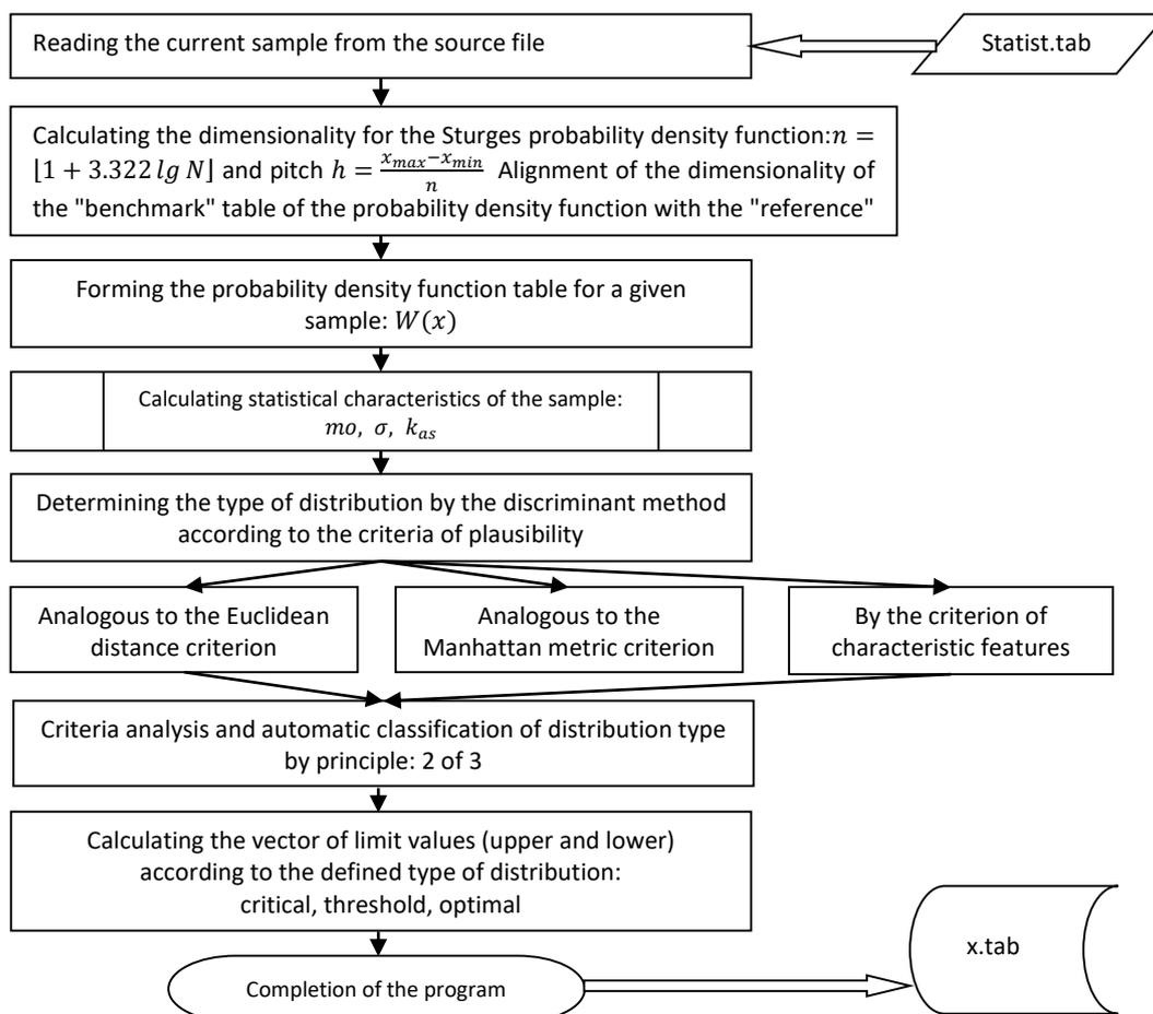
**Figure 3.** The Structure of the Digitization Program to Determine the Vector of the Limit Values of Safety Indicators
