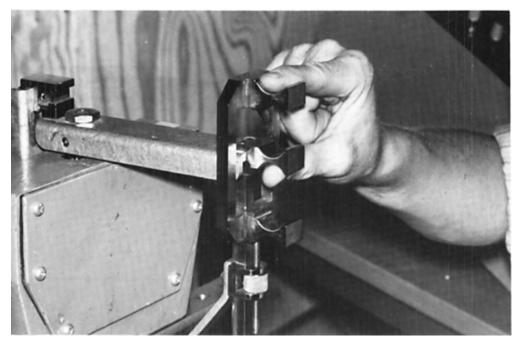
Fig. 1. To the left the pressduktor with the lever and the tightening screwnuts; to the right the adjustable finger grip.
