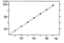
Fig. 4 a. The linearity on application of force (pull o, push  $\bullet$ ) to the press-duktor.
