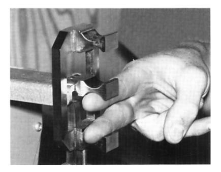
Fig. 3. Grip for measurement of the strength on opposition between digits I and II. The width of the grip is adjusted by means of the screw.
