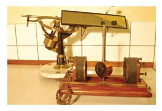
Figure 1. The equipment Holmgren used when he detected the retina current. The apparatus belongs to the Museum of Medical History in Uppsala.
