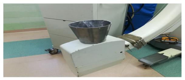
Figure 3. Fluoroscope tube with designed lead connector.
