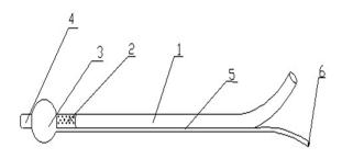
**Figure 1.** Sketch of the new catheter. The perimeter of the catheter is 14mm and the tip $\square$  is a closed end. There is a Non-return Valve $\square$  at the end of channe $\square$ .
