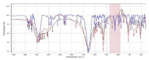
**Figure 3.** FTIR of the cultivated nanobacteria from positive samples (blue line) and the apatite kidney stone (black line). The peaks in 1000 to 1200 cm<sup>-1</sup> range belong to phosphate absorption and the stretching bond of phosphate in the structure of the mineralized shell. FTIR spectra of the negative sample are shown with the red line. The peaks in 1000 to 1200 cm<sup>-1</sup> range are absent (highlighted zone).
