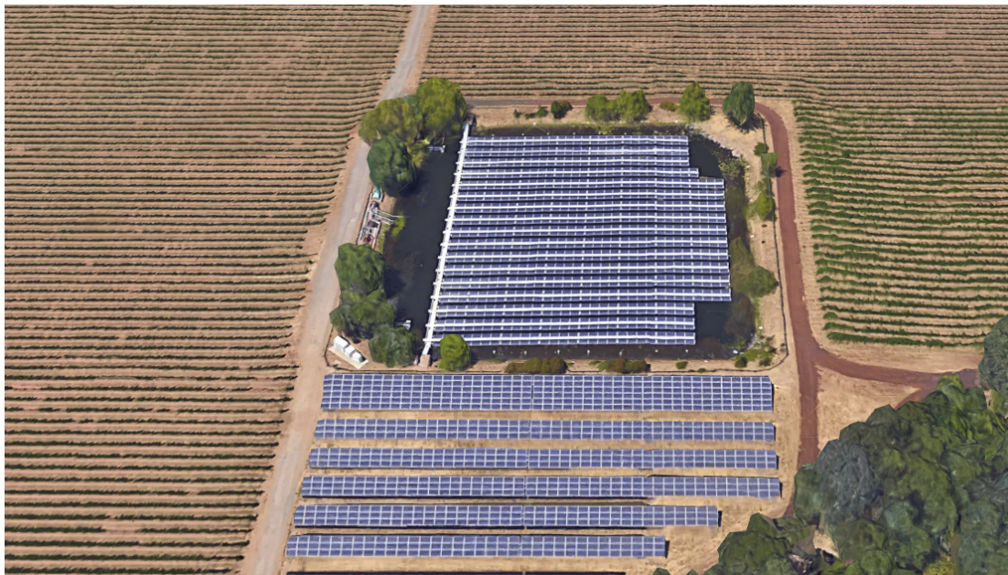
Figure 3. Ground-mounted and floating solar plants in Far Niente Winery, Oakville, California. Source: Google maps.
