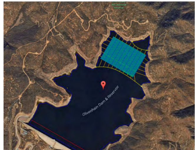
Figure 5. Olivenhain Reservoir and Dam in San Diego, California and floating solar plant layout in initial design. Source: Google Maps and San Diego County Water Authority.
