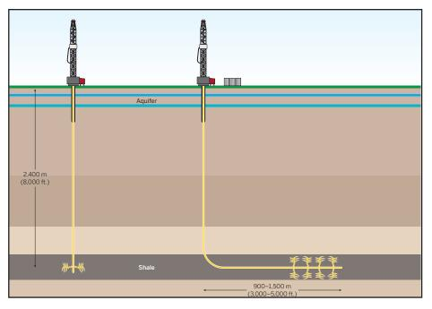
**Figure 2.** The figure shows examples of horizontal and vertical wells. A horizontal well is developed by drilling a vertical well thousands of meters into the ground then turning the drill horizontally into the zone from which the operator would like to produce hydrocarbons. The graphic is not to scale. (Graphic created by Jeff Phillips.)
