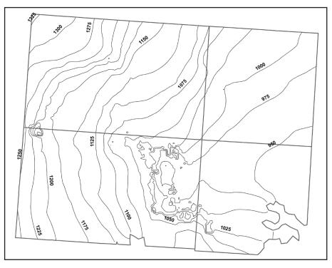
Figure 5. Predicted groundwater levels for the baseline by year 2060 (meters above mean sea level).
