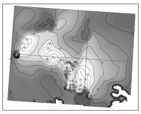
Figure 6. Grid image and contour lines for predicted groundwater drawdown (meters) for the baseline by year 2060.
