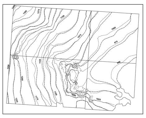
Figure 11. Comparison of predicted groundwater levels for baseline (solid lines) and Policy #3: Biotechnology (dotted lines) by year 2060 (meters above sea level).
