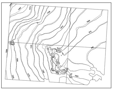
**Figure 7.** Comparison of predicted groundwater levels for baseline (solid lines) and Policy #1: Permanent conversion to dryland (dotted lines) by year 2060 (meters above sea level).
