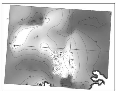
Figure 12. Grid image and contour lines for predicted groundwater drawdown (meters) for Policy #3: Biotechnology by year 2060.
