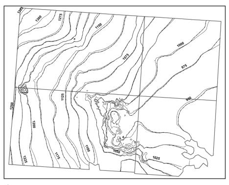
Figure 9. Comparison of predicted groundwater levels for baseline (solid lines) and Policy #2: Temporary conversion (dotted lines) by year 2060 (meters above sea level).
