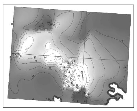
Figure 8. Grid image and contour lines for predicted groundwater drawdown (meters) for Policy #1: Permanent conversion by year 2060.
