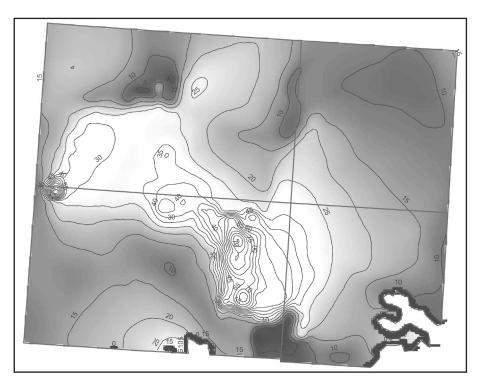
Figure 10. Grid image and contour lines for predicted groundwater drawdown (meters) for Policy #2: Temporary conversion by year 2060.
