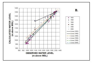
Figure 6. Calibration results for the exploitation period showing correlation between observed and calculated water levels.
