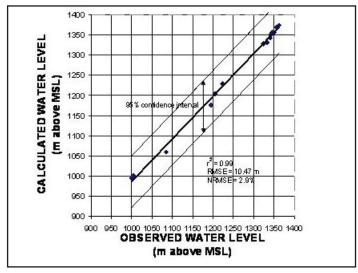
**Figure 5.** Calibration results for the predevelopment period (before 1950) showing 95% confidence interval and main statistics.
