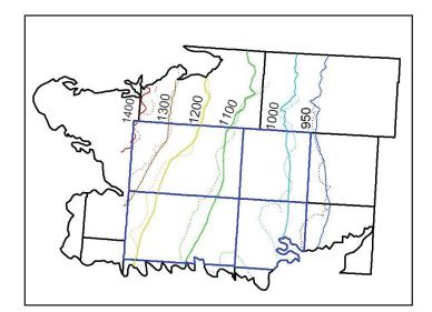
**Figure 4.** Historical (continuous lines) and simulated (dotted lines) groundwater levels (meters above the mean seal level) after calibrating for the predevelopment period.
