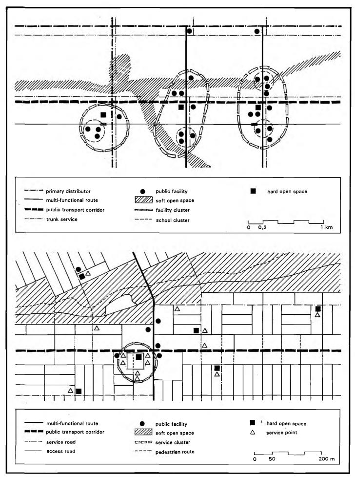
FIGURE 4: Conceptual diagram illustrating the spatial implications of the recommended layout planning principles at the sub-metropolitan and local scales
