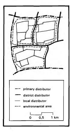
FIGURE 3: Conceptual diagram illustrating the "environmental area".
