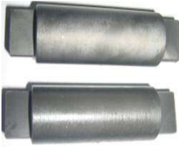
Figure 2. Brugger impact test specimen
