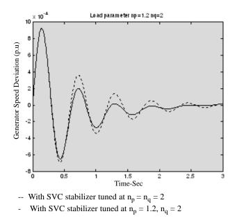
Figure 7. The system dynamic response at load parameters  $n_p=1.2$ ,  $n_q=2$  for 5% change in  $T_m$
