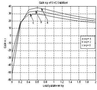
Figure 11. The computed SVC stabilizer gain  $K_p$  at different load model parameters
