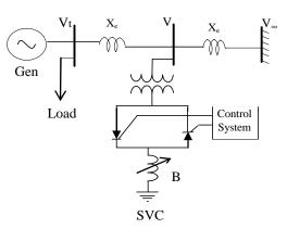
Figure 1. Power system single-line diagram
