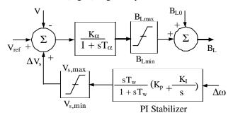
Figure 2. Block diagram of SVC with PI stabilizer
