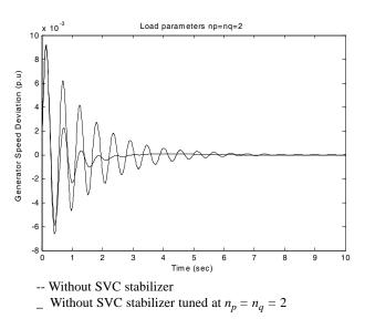
Figure 4. The system dynamic response at load parameters  $n_p = n_q = 2$  for 50% change in  $T_m$
