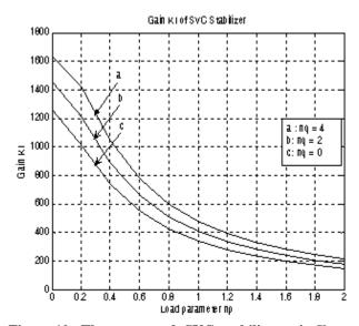
Figure 10. The computed SVC stabilizer gain  $K_1$  at different load model parameters
