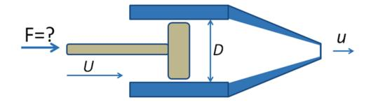
Figure A-1. Dimension and velocity direction of the nozzle.
