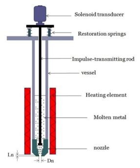
Figure 1. Schematic of the fabricated generator.
