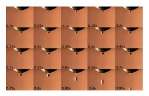
Figure 6. Photograph of metal droplet ejected from nozzle.
