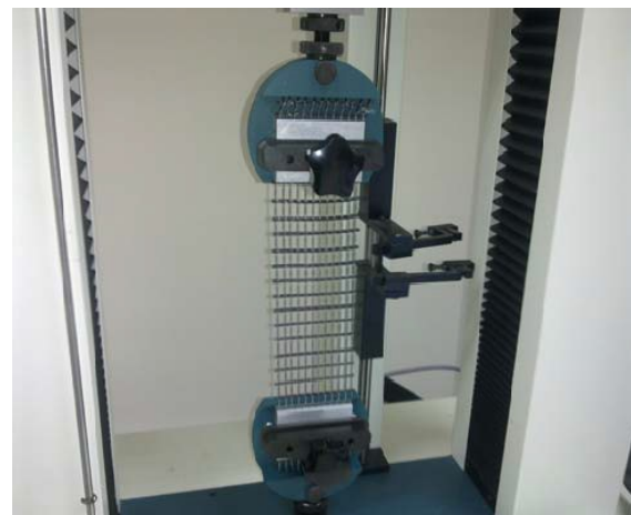
Figure 3. Photograph of pure tensile tests of textile specimens.
