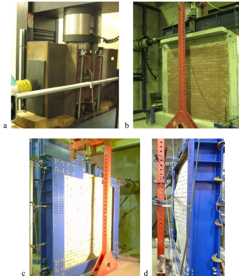
Figure 4. Experimental tests on SIM, with a) Displaying a friction test, b) An in-plane cyclic test on a type 3 panel, c) An in-plane cyclic test on type 1 and 2 panels, and d) An out-of-plane test.
