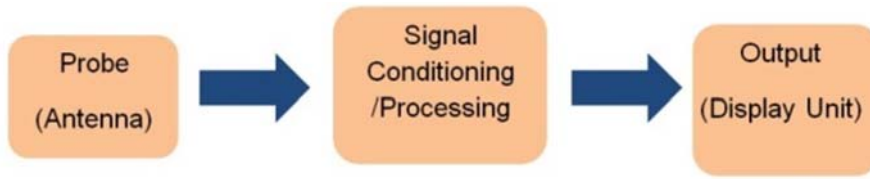
Figure 1. Block diagram showing the stages of the EM field detector circuit.
