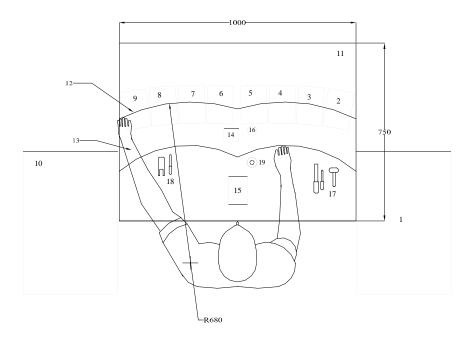
Legend: 1. Incoming bin (600x400); 2. Arc chutes bin (140x110); 3. Terminal clamp bin; 4. Tripping lever bin; 5. Cover parts bin; 6. Handle springs and long screws bin; 7. Handle and handle base bin; 8. Line terminal bin; 9. 3-pole body bin; 10. Outgoing bin (600x400); 11. Assembly table; 12. Maximum reach; 13. Normal reach; 14. Fixture; 15. Assembly area; 16. Grease container; 17. Tool area 1; 18. Tool area 2; 19. Power screwdriver.
