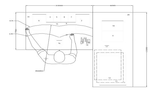
Legend: 1. Incoming bin (600x400); 2. Terminal lever bin (320x205); 3. Terminal clamp bin (140x110); 4. 3-pole body bin; 5. Handle base bin; 6. Handle springs, long screws, cover parts bin; 7. Handles bin; 8. Tripping lever bin; 9. Tripping lever springs bin; 10. Chutes; 11. Covers bin; 12. Outgoing bin; 13. Maximum reach; 14. Normal reach; 15. Grease container; 16. Assembly area; 17. Fixture; 18. Tool area; 19. Assembly table; 20. Side table; 21. Power screwdriver.
