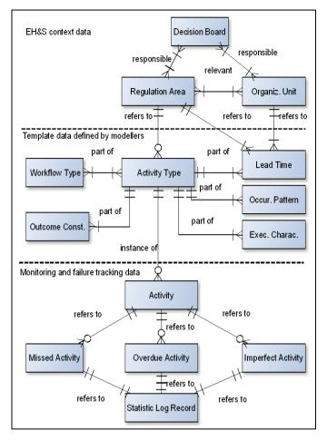
Fig. 1. Proposed workflow meta data model.
