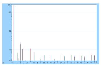
Fig. 9. Spectrum of harmonic voltage of higher levels with designated permitted limits in accordance with CSN EN 50160-BPS2
