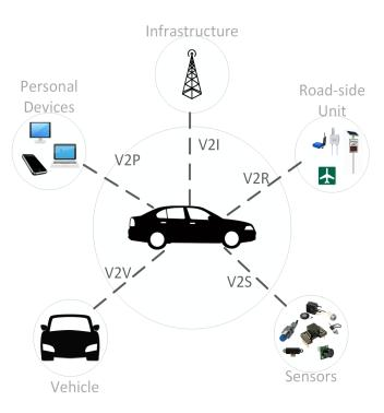
Fig. 4. Types of IoV communication, based on [31].
