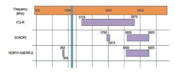
Fig. 9. Spectral range for ITS applications [55].
