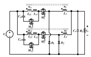
Fig. 10. Interleaved coupled-buck converter with active-clamp circuits [15].
