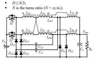
Fig. 9. Interleaved DC–DC high step-down buck converter with winding-crosscoupled inductors (WCCIs) and passive-lossless clamp scheme [14].
