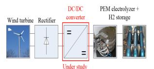
Fig. 2. Hydrogen generation pathways from wind turbines.
