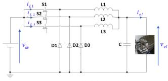
Fig. 3. IBC connected with the electrolyzer.
