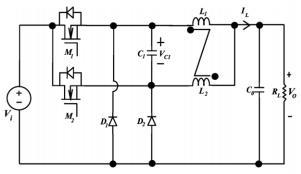
Fig. 4. IBC with a single-capacitor snubber [9].
