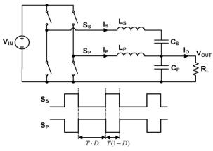
Fig. 8. Stacked interleaved topology and timing chart [13].
