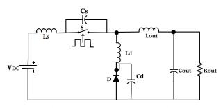
Fig. 3 Circuit Diagram of Quasi Resonant Buck Converter
