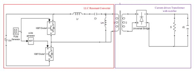
Fig. 2 Simulink block diagram of current mode control of LLC resonant converter
