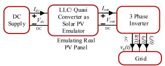
Fig. 1 PV emulator connection to a grid connected 3 phase inverter.
