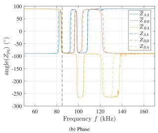
Fig. 4. Magnitude and phase of impedance matrix entries as a function of frequency: 1) solid curves – measurements  $\overline{Z}_{pq}(f_{\nu})$ ; and 2) dashed curves – model  $Z_{pq}(f_{\nu},\mathbf{p}_0)$  for the initial parameter vector  $\mathbf{p}_0$ . The vertical dashed line show the operating frequency 85 kHz.
