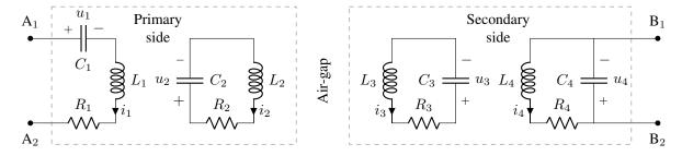
Fig. 2. Circuit diagram for the magnetically coupled resonators with four coils and capacitors.
