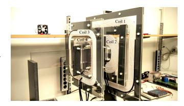
Fig. 1. Photo of the air-wound coils used in the WPT system prototype with four magnetically coupled resonators.
