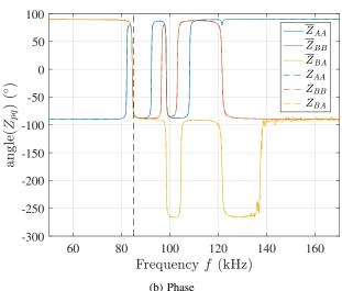
Fig. 6. Magnitude and phase of impedance matrix entries as a function of frequency: 1) solid curves – measurements  $\overline{Z}_{pq}(f_{\nu})$ ; and 2) dashed curves – model  $Z_{pq}(f_{\nu}, \mathbf{p}^*)$  for the optimized parameter vector  $\mathbf{p}^*$ .
