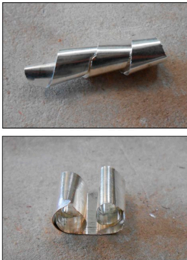
Figure 2. Cornet (top) and volute shapes (bottom) in the same rolled cupellation bead.
