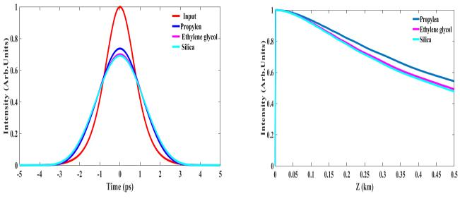
**Figure 4.** The difference in amplitude of different core materials with respect to time.
