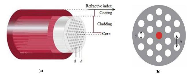
Figure 1. (a) Longitudinal section of the photonic crystal fiber, (b) Cross-section of the photonic crystal fiber.
