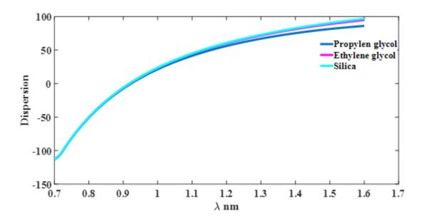
Figure 3. The dispersion of cores consisting of SiO<sub>2</sub>, C<sub>3</sub>H<sub>8</sub>O<sub>2</sub>, and C<sub>2</sub>H<sub>6</sub>O<sub>2</sub>.
