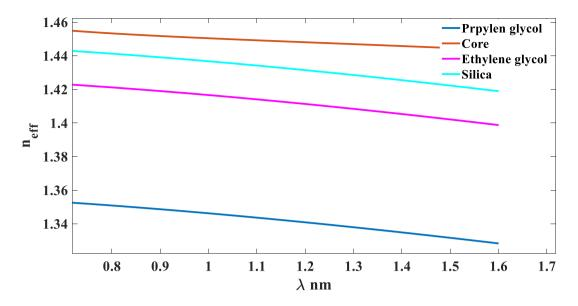
**Figure 2.** The relationship between the refractive indices of  $SiO_2$ ,  $C_3H_8O_2$  and  $C_2H_6O_2$ .
