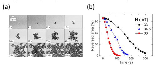
**Figure 3.** Time-dependent magnetization (a) MOKE images of 10  $\mu$ m × 11  $\mu$ m captured after applying a magnetic field of 33 mT. (b) Reversed area of the magnetic domains versus time curves plotted after the application of various reverse magnetic fields.
