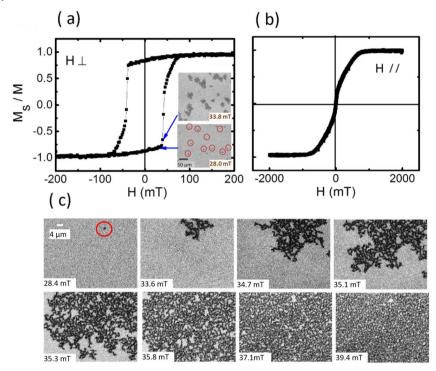
**Figure 2.** (a) Hysteresis loops of  $(Co/Pt)_{12}$  MLs in the out-of-plane direction. The 300 µm × 300 µm using × 4 objective lens MOKE images (insert) of the magnetic domains' nucleation were taken in the beginning of the evolution (b) Hysteresis loops of  $(Co/Pt)_{12}$  MLs in the plane to the surface of the film. (c) MOKE images of magnetic domains' evolution with the magnetic field using × 40 objective lens; the field was increased in steps of 0.01 mT/s.
