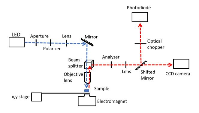
Figure 1. A schematic drawing of the MOKE microscope set up.
