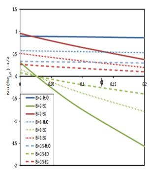
**Figure 28.** Nusselt number for different values of Bi and  $\varphi$  in Cu- $H_2O$ , Cu-EG, and Cu-EO nanofluids.
