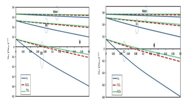
**Figure 32.** Nusselt number for different base fluids using different nanoparticles when Bi = 0.5.
