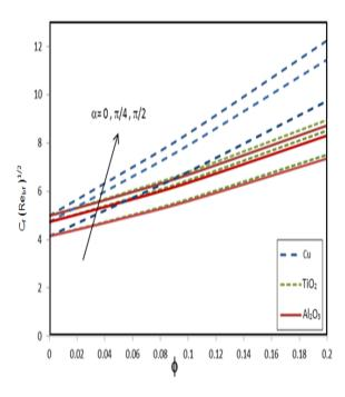
**Figure 40.** Skin-friction coefficient for water based nanofluid for different values of  $\alpha$ .
