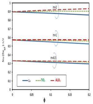
**Figure 29.** Nusselt number for different values of m and  $\varphi$  in Cu- $H_2O$ ,  $TiO_2$ - $H_2O$ , and  $Al_2O_3$ - $H_2O$  nanofluids.
