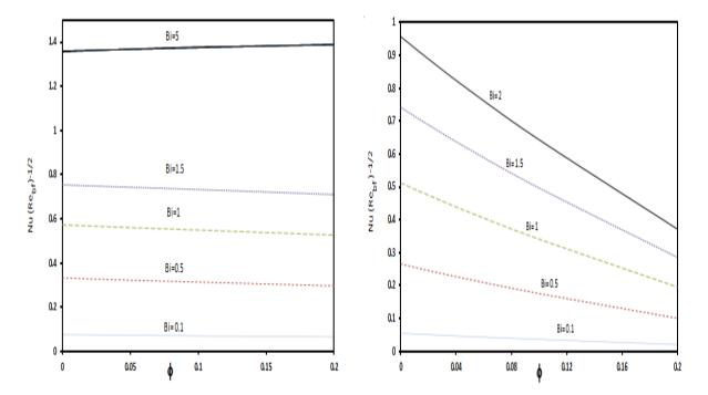
**Figure 24.** Nusselt number for different values of Bi and  $\varphi$  for Cu- $H_2O$  nanofluid.
