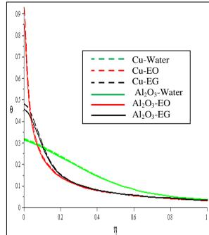
**Figure 20.** Velocity profiles for comparison between Cu and  $Al_2O_3$  nanoparticles in different base fluids.
