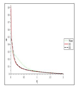
**Figure 18.** Temperature profiles in different base fluids with Cu nanoparticles.
