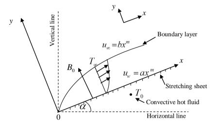
Figure 1. Flow configurations and coordinate system.
