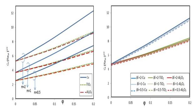
**Figure 38.** Skin-friction coefficient for water based nanofluid for different values of m.
