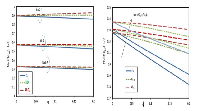
**Figure 30.** Nusselt number for different values of Bi and  $\varphi$  in Cu- $H_2O$ ,  $TiO_2$ - $H_2O$ ,  $Al_2O_3$ - $H_2O$  nanofluids.
