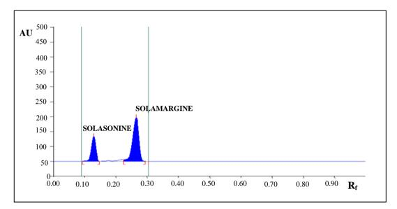
Figure 2. HPTLC chromatogram of solasonine ( $R_f 0.13$ ) and solamargine ( $R_f 0.27$ ) 1000 ng/spot each at 530 nm.
