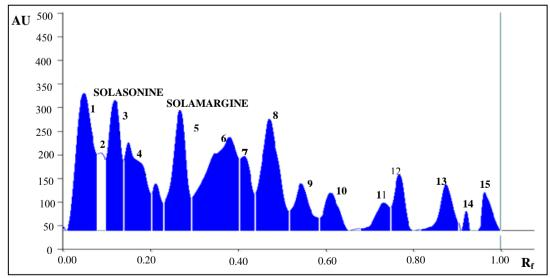
**Figure 3.** HPTLC chromatogram of Sample at 530 nm, using solvent system Chloroform: Methanol: 5% Ammonia (7: 3: 0.5) showing the presence of solasonine and solamargine.
