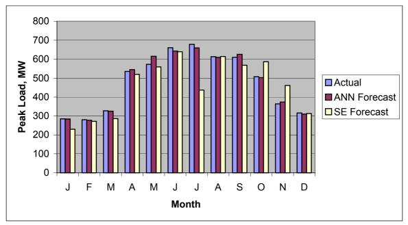
**Figure 2.** Actual and forecasted results for the load model.
