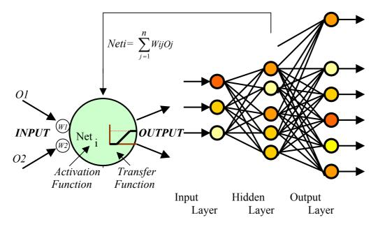
**Figure 1.** A typical back-propagation architecture.
