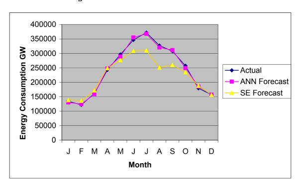
**Figure 3.** Actual and forecasted results for the energy consumption model.
