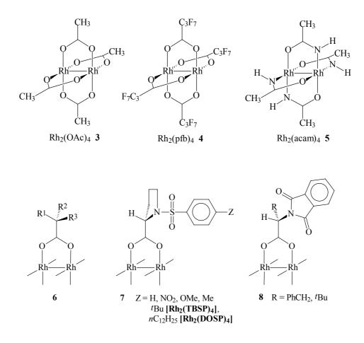
Dirhodium(II) perfluorobutyrate,  $Rh_2(pfb)_4 4$ , is the most reactive dirhodium(II) catalyst, and its selectivity in diazo decomposition reactions is often correspondingly poor (Doyle *et al*, 1993b). In contrast, dirhodium(II) carboxamidates such as  $Rh_2(acam)_4 5$ , which have two nitrogen and two oxygen donor atoms at each rhodium, with the two nitrogens arranged *cis* to each other (a [2,2-*cis*] configuration)
