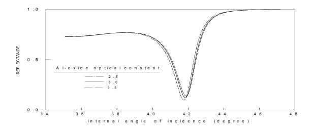
**Figure 3.** The calculated reflectance as a function of incidence angle for different Al-oxide optical constant. The wavelength is 633 nm. The air gap, Al-oxide and Al thickness are 650 nm, 3.4 nm and 22 nm respectively.
