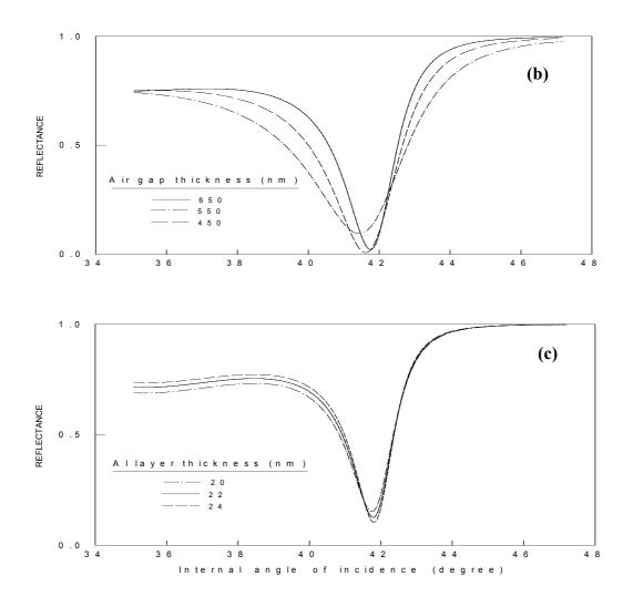
Figure 2. The calculated reflectance as a function of incidence angle for different:
