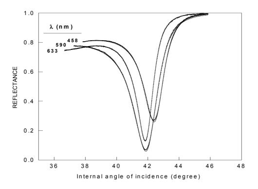
**Figure 5.** Fit of the measured ATR (dots) to the calculated reflectance (line) as a function of the internal angle of incidence for different wavelengths. Fitting and invariant parameters are shown in table 1.
