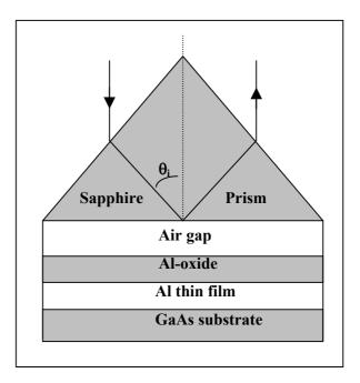
Figure 1. Detail of arrangement for making Otto configuration ATR measurements on Al / GaAs sample.
