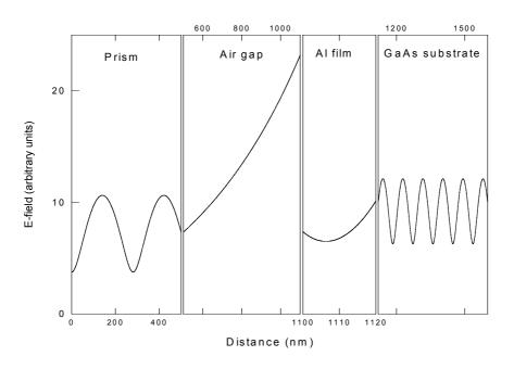
**Figure 4.** The calculated E-field as a function of distance in each medium of the geometry Prism / Air gap / Al / GaAs, at resonance angle  $\theta_i = 41.8^\circ$  and wavelength  $\lambda = 633$  nm.
