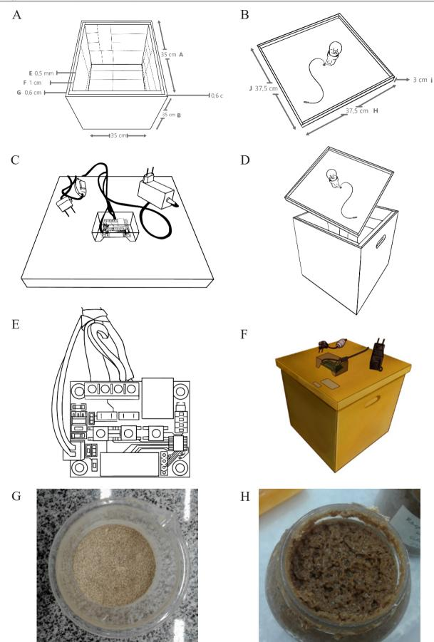
Fig 1. Details of the constitution of the artisanal incubator: A. Styrofoam and polyethylene lined box; B. cover with socket and lamp; C. thermostat and socket; D. Inner face of box and lid; E. digital thermostat; F. ready incubator; G. diet before fermentation and H. fermented diet.
