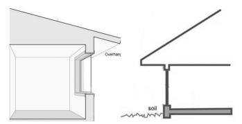
Fig 1. Schematic of roof overhang commonly used for built structures in the Philippines.
