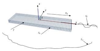
Figure 1. Fluid boundaries and Coordinate system
