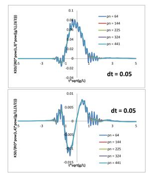
Figure 16. Nondimensional exciting heave and pitch IRFs of Wigley hull form at Fn = 0.2 and  $\beta = 180^{\circ}$
