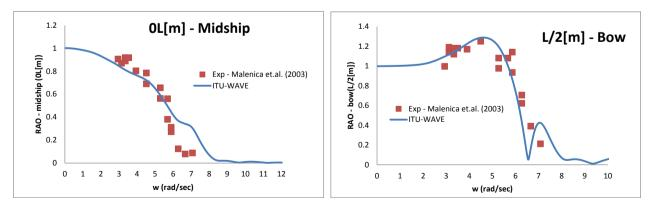
Figure 13. Vertical RAOs of flexible barge at mid-ship (0) and bow (L/2) with heading angle  $\beta = 180^{\circ}$ , Fn=0.0 and stiffness factor  $S = EI/\rho gL^5 = 1.99 \times 10^{-4}$
