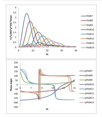
**Figure 7.** Nondimensional exciting force amplitudes and phase angles of elastic slender barge for the first 8 deformable modes including 7, 8 and 9 modes
