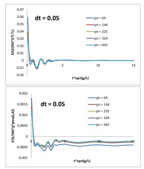
Figure 15. Nondimensional radiation heave and pitch IRFs of Wigley hull form at Fn = 0.2
