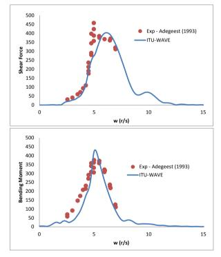
**Figure 18.** Shear force and bending moment of Wigley hull form at Froude number Fn = 0.2 and heading angle  $\beta = 180^{\circ}$  using 8 free-free Euler-Bernoulli elastic beam modes
