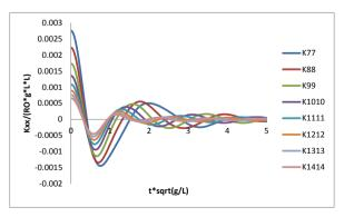
Figure 4. The first 8 deformable modes of nondimensional radiation IRFs of the elastic barge
