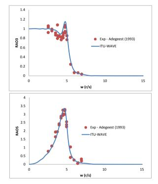
Figure 17. Heave and pitch RAOs of Wigley hull form at Fn = 0.2 and  $\beta = 180^{\circ}$
