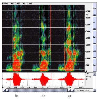
Figure 1. Spectrogram of the syllables /ba/, /da/ and /ga/.
