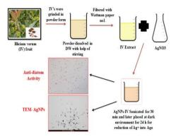
Fig. 2. Schematic route of AgNPs formation using plant extract of illicium verum (IV).
