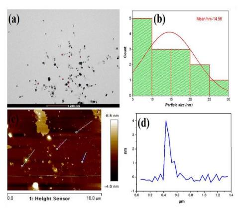
Fig. 7. Transmission electron microscopy image at 200 nm (a), particle size distribution through TEM image (b), atomic force microscopy image (c), and Particle size obtained through AFM image (d) of AgNPs-I
