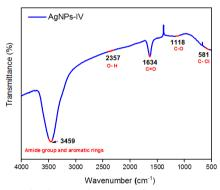
Fig. 4. FTIR Spectrum of AgNPs-IV.
