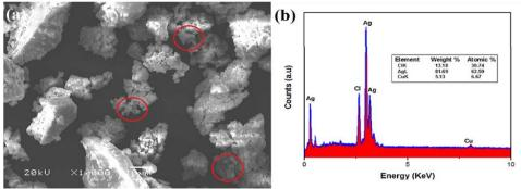
Fig 6. Scanning electron microscopy image of AgNPs-IV (a), EDX Spectrum of AgNPs-IV (b).
