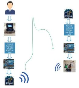
Fig. 1. Proposed System block diagram.
