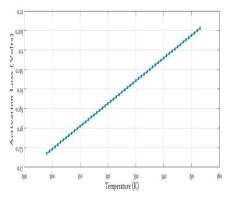
Fig. 5. The impact of temperature on activation losses.
