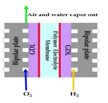
Fig. 2. Flow channels and flow directions [5].
