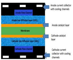
Fig. 1. PEM Fuel Cell diagram [3].
