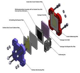
Fig. 3. Exploded view of PEM Fuel cell [16].
