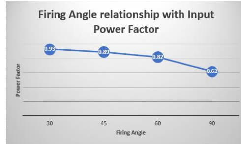
Fig. 18. Relationship of Firing angle and Input Power Factor.
