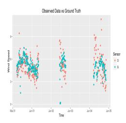
**Figure 7**: Observed data from ultrasonic anemometer vs ground truth data from NRG 40H
