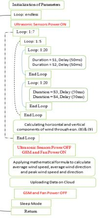
Figure 6: Software flow of advance vision of ultrasonic anemometer
