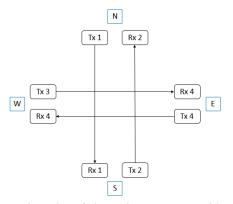
Figure 1: Design of ultrasonic anemometer with four modified HC-SR04
