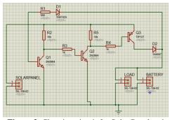
Figure 3: Charging circuit for Solar Panel and lithium-ion battery
