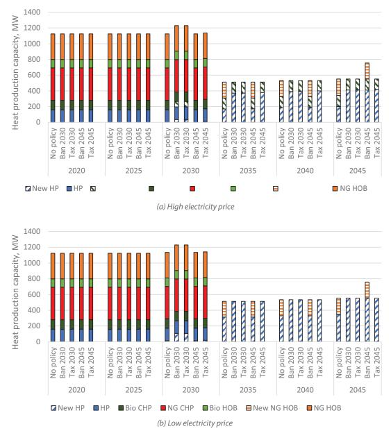
Figure 5 Capacity of DH supply plants. EH and MSW incineration remain unchanged and have been left out in the figures to improve readability. Also, oil HOB and electric HOB available from the starting year but are never utilized are left out to improve readability.
