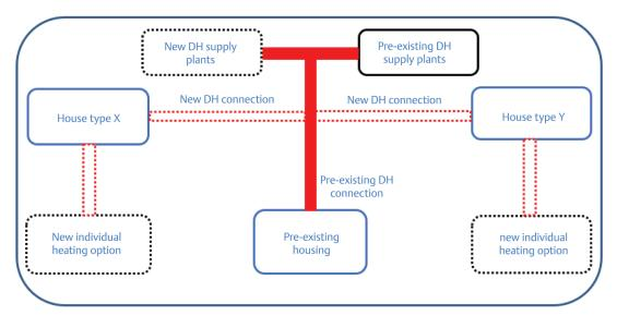
Figure 2. Schematic representation of the model setup for determining the cost optimal heating solution with different types of new housing.
