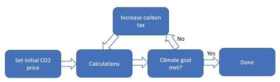
Figure 1. Iterative method for determining carbon tax required to phase out fossil fuel use at a specific year when using an increasing carbon tax policy
