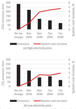
Figure 6 Increase of total system cost and CO2 emissions for the local heating system for entire modelling period by introduction of different climate policies.
