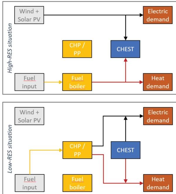
Figure 3: CHEST integrated in a CHP-based DH supply system in a situation with high production of wind and solar power (top) and one with low production (bottom).
