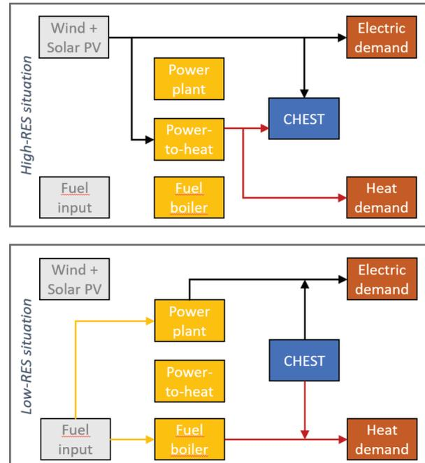
Figure 4: CHEST integrated in an electrified DH supply system in a situation with high production of wind and solar power (top) and one with low production (bottom).
