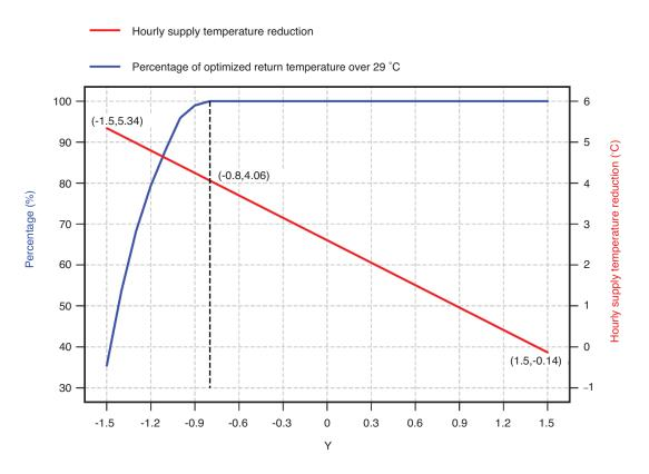
Figure 6: The hourly supply temperature reduction on simulation period and the percentage of predicted return temperature above the defined minimum return temperature (29°C) with different optimization strategies
